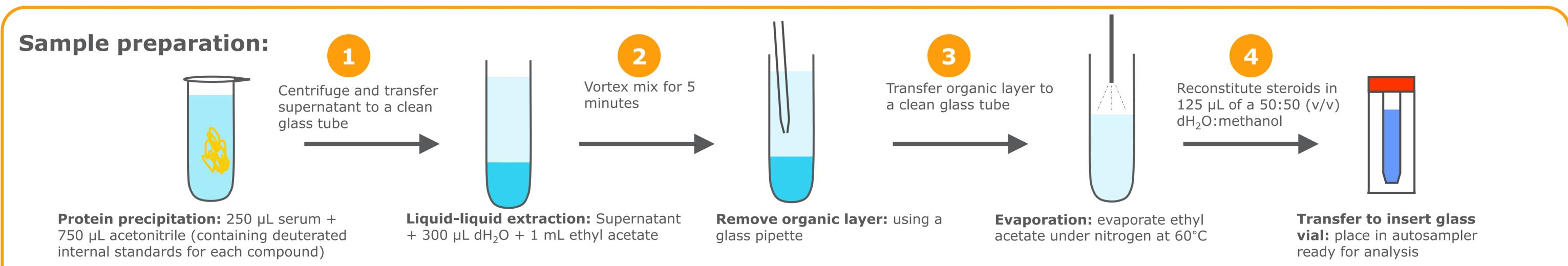
• Schematic of sample preparation for LC-MS/MS. Each step has been extensively optimised to maximise recovery and minimise ion suppression. Combining protein precipitation with liquid-liquid extraction results in reproducible extraction across the range of the polarities of the steroids quantified.
