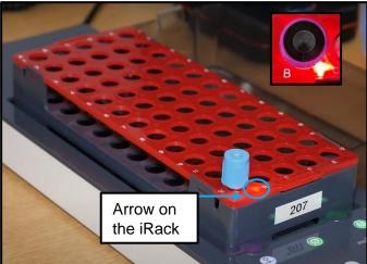
5. You have 2-3 seconds to place the sample tube into the iRack. The arrow on the rack shows the marked tube.
