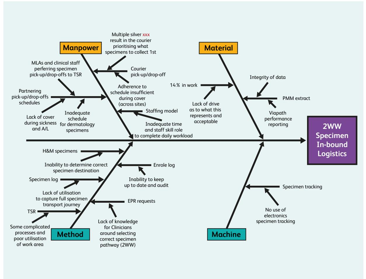
Example of Fishbone diagram to illustrate investigation root causes
